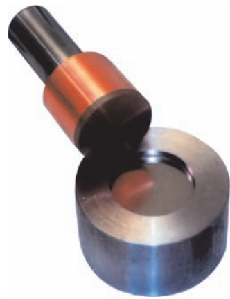
Mirror machining: Ra0.15 μm
