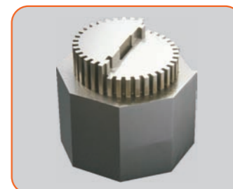
Application 8 Material : Cr12 Brass wire Φ0.25mm Cutting times : 3
