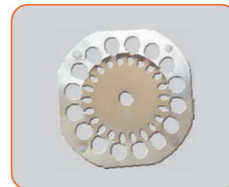
Application 6 Material : Cr12 Brass wire Φ0.25mm Cutting times : 3
