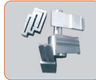
Application 1 Material : Cr12 Brass wire Φ0.2mm Cutting times : 3
