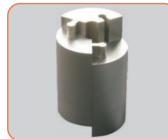
Application 5 Material : Cr12 Brass wire Φ0.2mm Cutting times : 3
