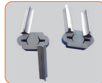
Application 4 Material : Cr12 Brass wire Φ0.25mm Cutting times : 3
